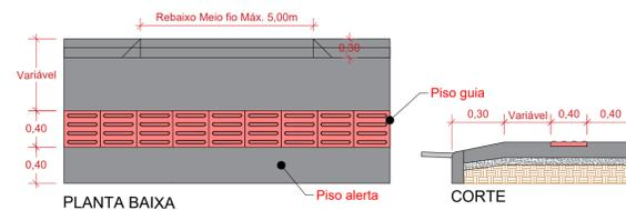
DETALHE REBAIXO MEIO FIO GARAGEM SEM ESCALA
