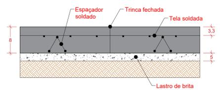
DETALHE PISO CONCRETO ARMADO SEM ESCALA
